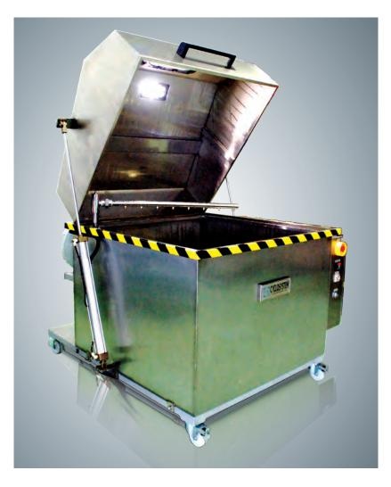
The Cyclojet INEX Series is probably one of the simplest and most popular ranges of automatic Spray Jet Cleaning Machines in the industry. As the names implies, the "INEX" series is an "INEXpensive" range of Jet Spray Cleaners - specially designed and developed for serial production and cater to the mass market to clean small parts automatically. It is possibly the answer to the general industrial cleaning needs as washing machines are highly common for most household nowadays.
